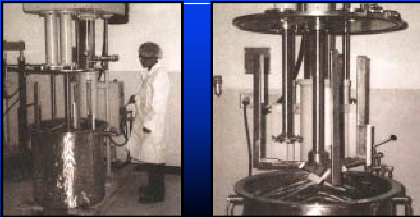
"50 gallon high speed disperser – produced by Applied Silicone Corp, Ventura, California"
